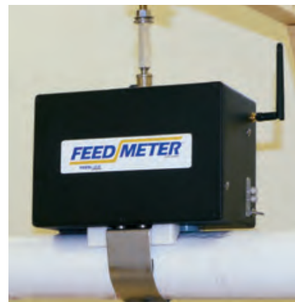
The new FeedMeter system allows measurement of feed flow through a standard feed line
