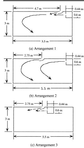
Figure 4 Arrangement of slot inlets
