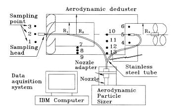
The drop in air velocity and pressure were measured using a hot wire anemometer. Air velocity was measured at all points shown in Figure 4 (numbered 1 to 13). Total pressure drop across the deduster was measured at points numbered 4, 5 and 6.
