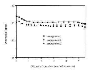
Figure 6 Effect of arrangement on the ammonia concentration along breathing line
