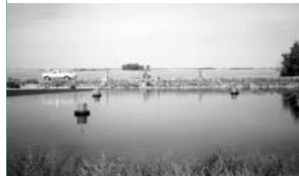
Figure 1. Gas collection and sampling system used to measure GHG emissions from manure storage facilities.
