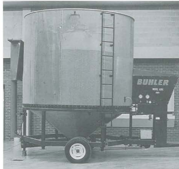
Grain dryers are used to reduce the moisture content of wet grains thus preventing spoilage.
