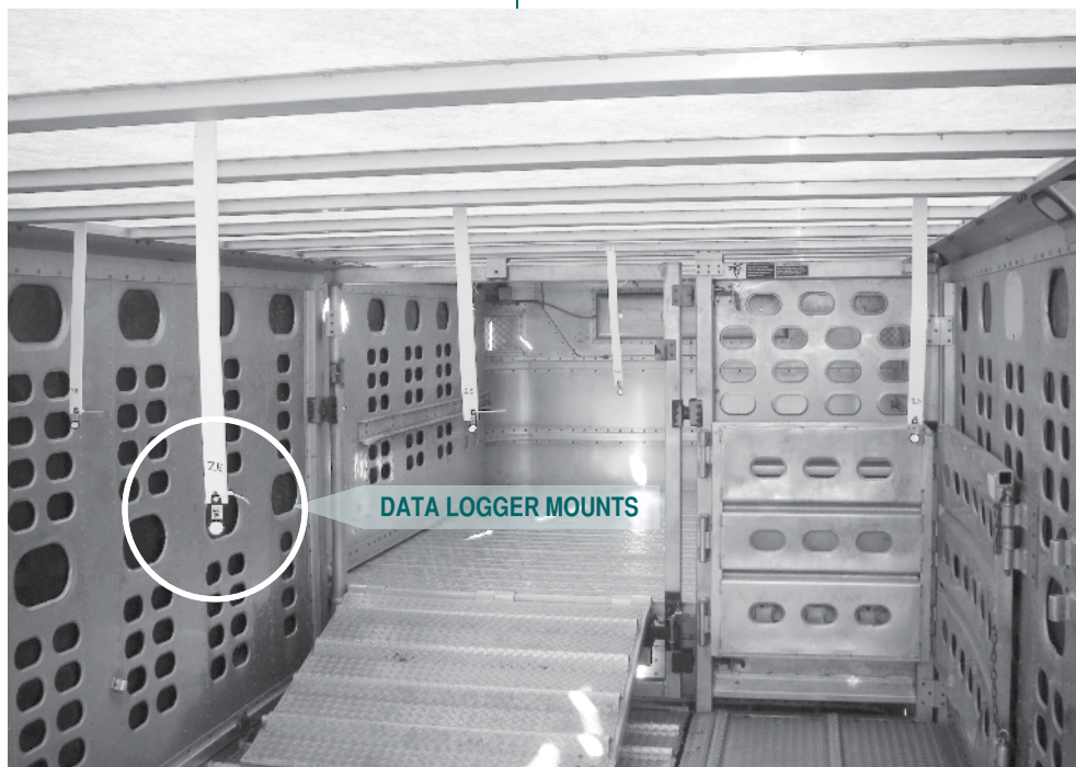
Figure 1. Placement of data loggers in the trailer (compartment 3).
