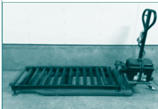
The low-cost deadstock mover is an innovation using a pallet jack, rollers and an electric winch
