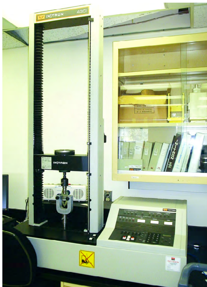
Figure 5. Tenderness was evaluated by the amount of force required to slice through a core of cooked meat (shear force) using an Instron Materials Testing System equipped with a Warner-Bratzler shear cell.
