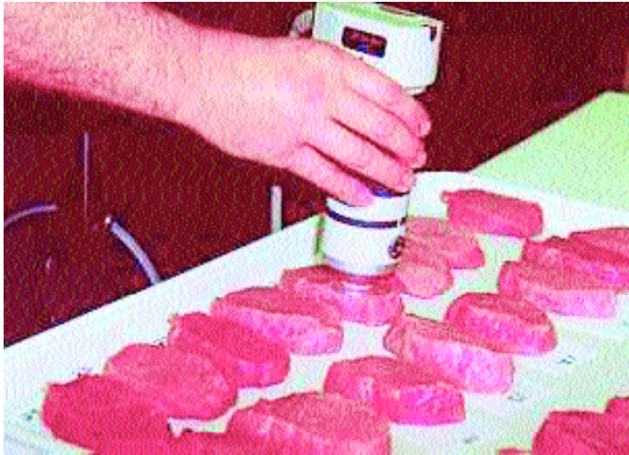
Figure 4. To measure light reflectance off the surface of the muscle, the Minolta CR-300 colour meter was placed in full contact with the chop, flashed a light beam and recorded four reflectance values.
