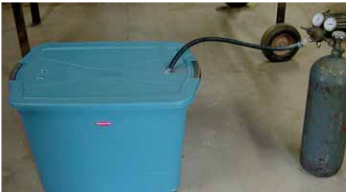
The CO 2 euthanasia device constructed by Jerry May, extension educator for Michigan State University.
