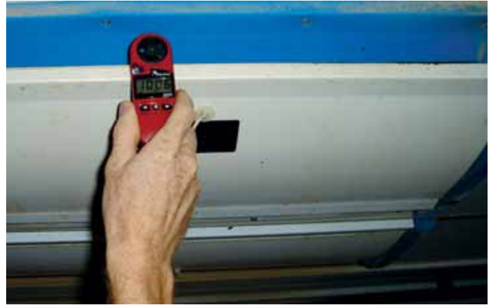
Figure 2: Using a Kestral model 3000 vanometer to measure inlet velocity. It measured 846 fpm in this photo
