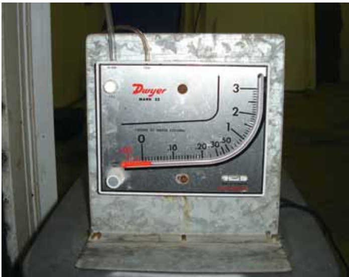
Figure 1: Manometer to measure static pressure
