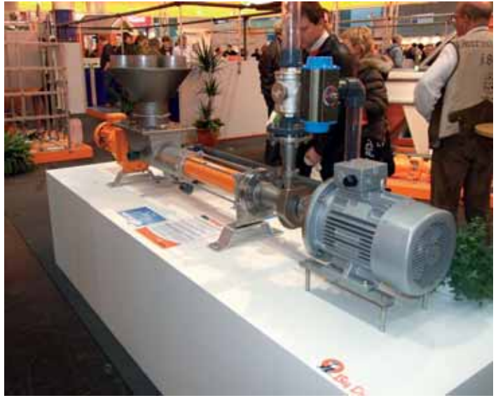
Big Dutchman's MixPump is a compact liquid feeding system which does away with the need for a mixing tank, agitator or weighing system.
