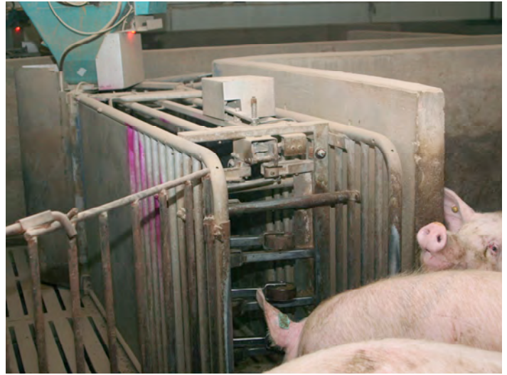
The Nedap electronic feeder: note the exit race that takes sows away from the feeding area once they have eaten
