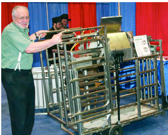
The egate portable sorter has a fold-up rear section making it easier to move around
