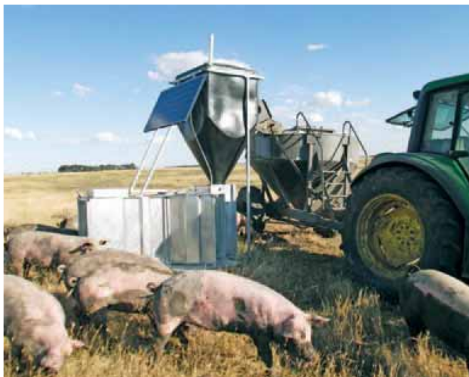
The Apollo solar powered electronic sow feeder in use at an outdoor pig unit
