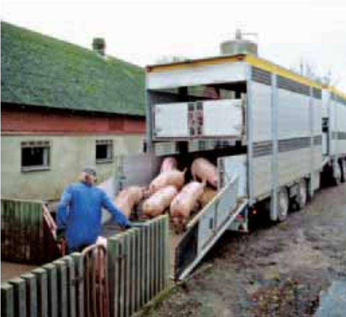
Pigs being loaded at a farm in Denmark – note that the top deck lowers so there are no ramps for pigs to climb
