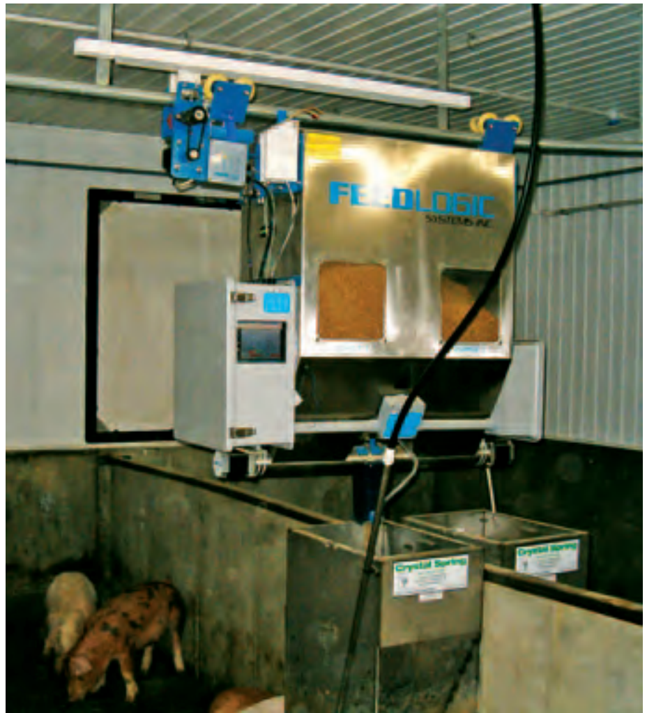
The FeedLogic feeder at the Drumloche trial barn delivers precise amounts of the required diet to individual pens
