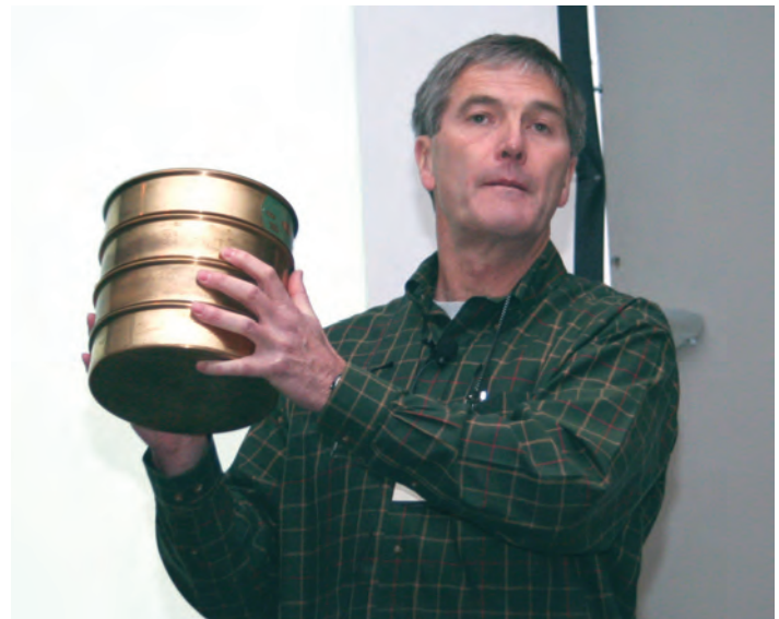
Jim Gowans, one of the founders of the workshop, demonstrates a 3-screen device for measuring feed particle size
