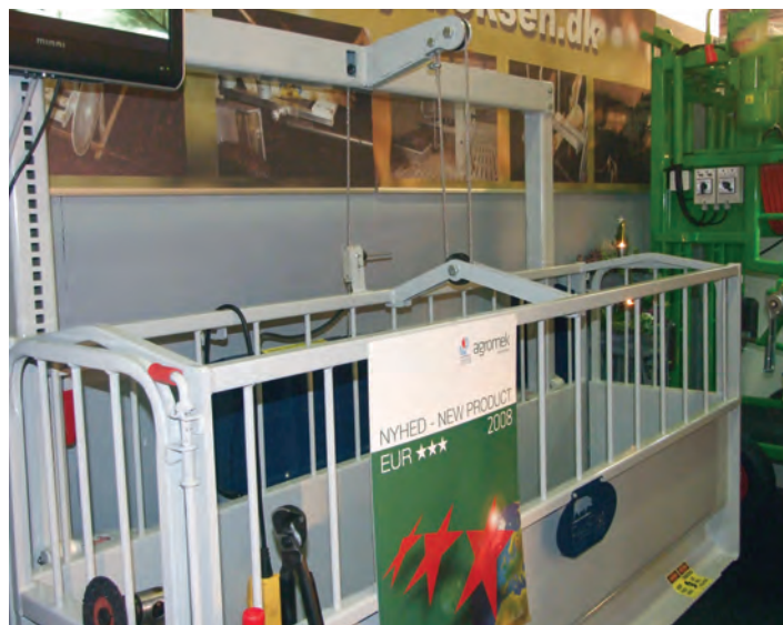
The FeetFirst trimming box hoists sows off the ground allowing feet trimming to take place
