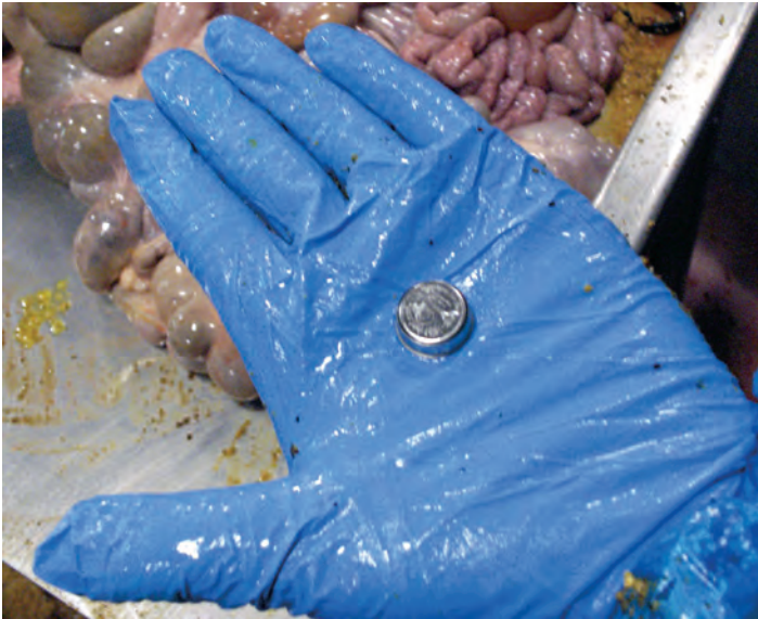
i-button temperature sensor after recovery from digestive tract of a pig
