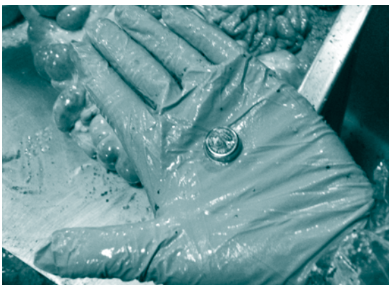
i-button temperature sensor after recovery from digestive tract of a pig.
