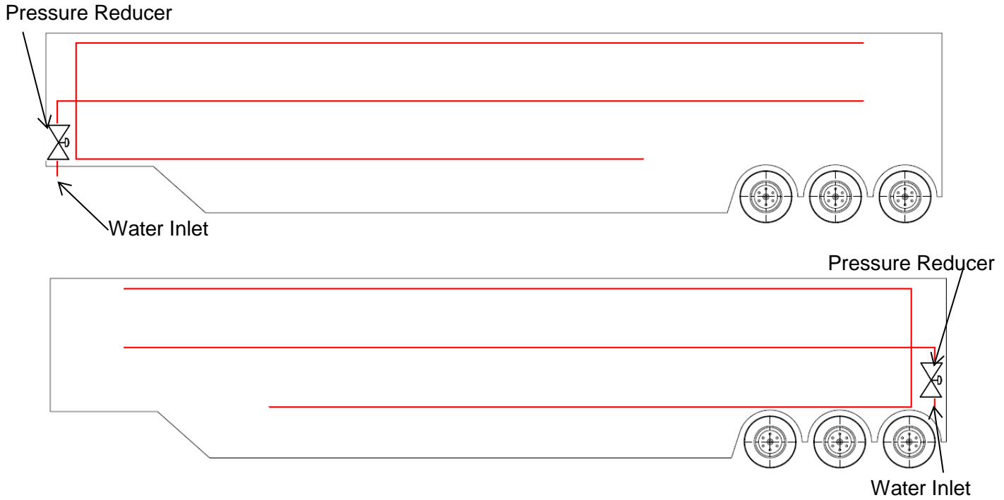
Figure 4 Possible layouts for water line configuration on one side and along the centreline of the trailer
