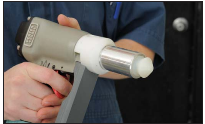
■ Zephyr-E gun in the fired position exposing the conical nylon bolt head.
