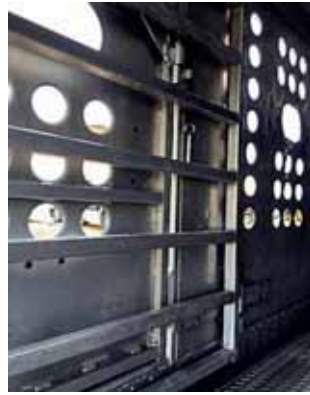
Figure 1. Merrit back gate, showing standard square cross bars.
