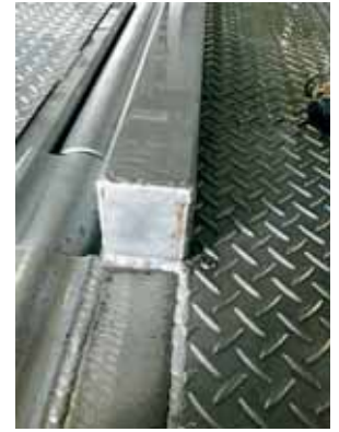
Figure 3. Many trailers put caps on exposed beams or rails to prevent buildup of bedding.
