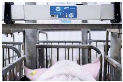
Above: Part of the PigWatch system mounted above a sow's stall. This portion contains the built-in motion sensors.
