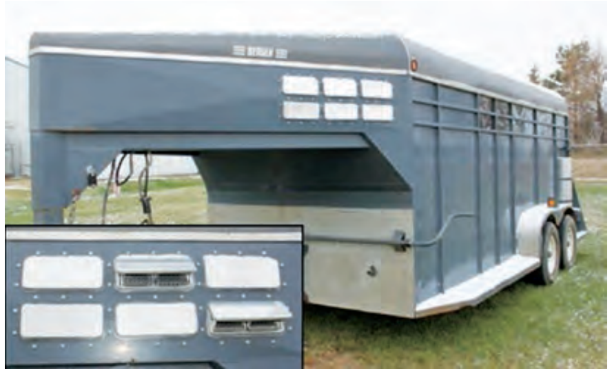
Figure 1. Commercial swine transport trailer with installed air inlets (inset) for the air filtration system.
