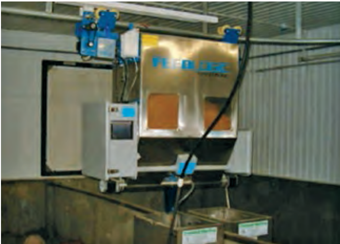
The intelligent feed delivery robotic system help to keep track of feed delivered to each pen accurately and on a daily basis. The robotic system manages multiple diets and can also blend feeds or dispense supplements or additives to specific pens with no cross contamination.
