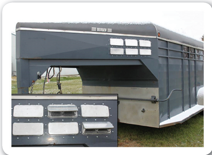
Figure 1. Commercial swine transport trailer with installed air inlets (inset) for the air filtration system.
