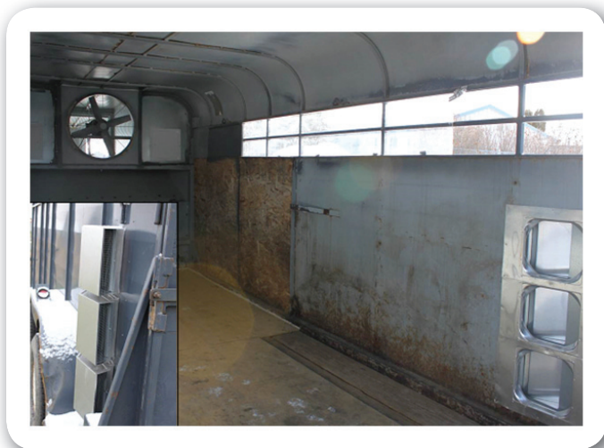
Figure 2. Ventilation fan and air filter holder were installed in gooseneck area which was partitioned from the animal compartment of the trailer. Exhaust vents (inset) were installed on both sides of the trailer.
