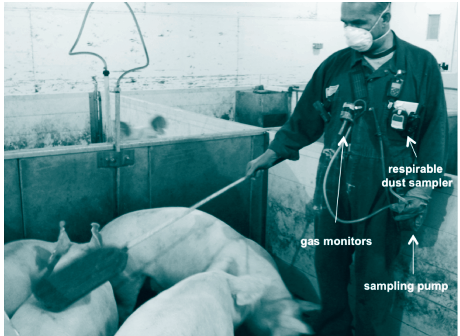
Figure 1. Gas monitors and respirable dust sampling gear worn by the worker while performing specific tasks during personal sampling.
