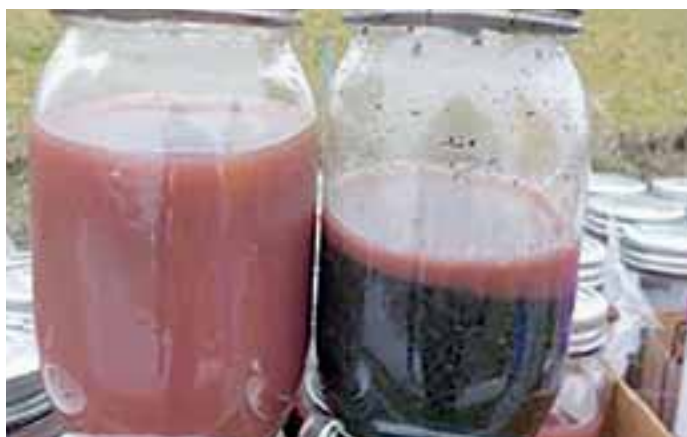
Manure samples from upper and lower lagoon depths contain different percentages of solids
