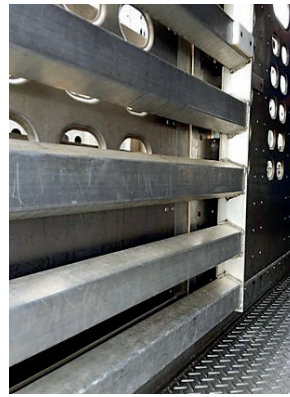
Figure 2. Eby back gate, showing slanted cross bars for greater ease of cleaning.
