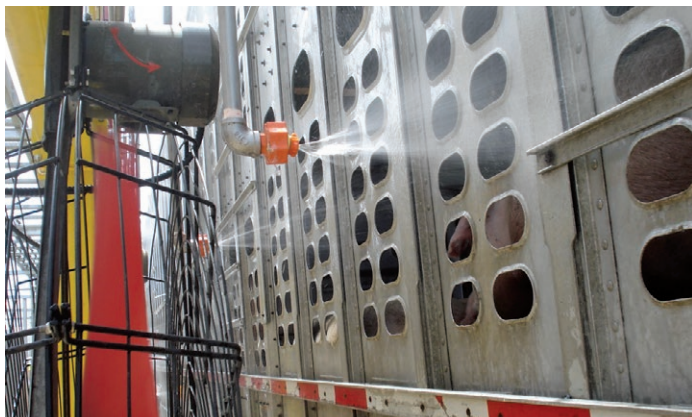
Combined water sprinkling and ventilation system. Source: Sherbrooke Research and Development Centre, AAFC
