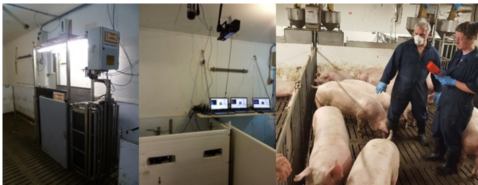
Figure 4. Vision systems (from left to right: Optisort, Kinect and PigWei)
