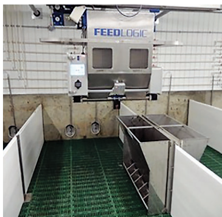
Feed Logic system. The automated feed delivery robotic system keeps track of feed delivered to each pen accurately. The robotic system manages multiple diets and can also blend feeds or dispense supplements or additives to specific pens with no cross contamination.
