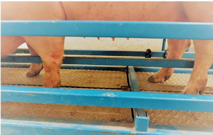
Force plate scale measures individual limb weight distribution while sow is standing still eating.
