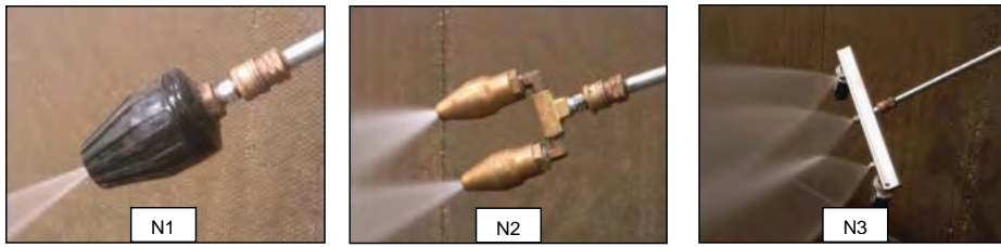
Figure 2. Four different types of pressure-washing nozzles used: conventional nozzle (N1), Y-nozzle (N2), water broom (N3), and 4-in-1 nozzle (N4).
