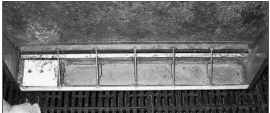
Figure 1 Feeder trough coverage with a gap adjustment providing a gap opening of 9.2 mm.
